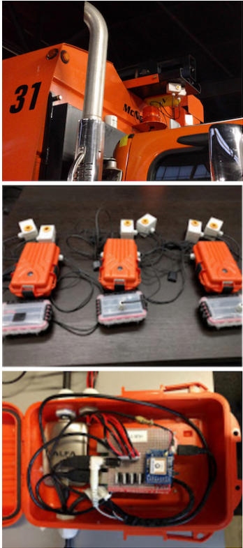
Figure 7: Cityscanner sensor modules prototype
