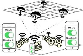
**Figure 1:** Symbolic sensor setup on the ceiling where the sensors were mounted together with lighting material. The sensors were equipped with directional antennas with free line of sight towards the visitors.
