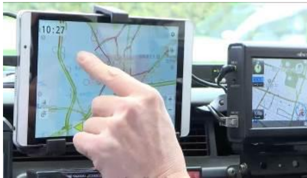
Figure 4: Taxi demand prediction visualization system. The system calculates future passenger boarding demands and visualizes them in real time on a tablet device screen. The tablet device is installed in the dashboard of taxis.
