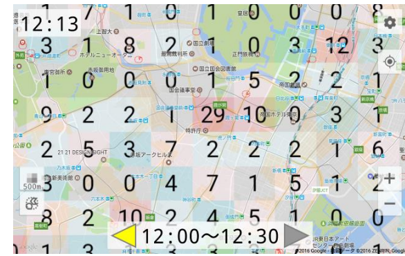
Figure 5: Output image of the taxi demand forecast system. The figures in each grid cell indicate expected the number of passengers boarding in a target 500-m mesh area in the next 30 min. Areas with high demand are colored in red and those with low demand are colored in blue or are transparent.
