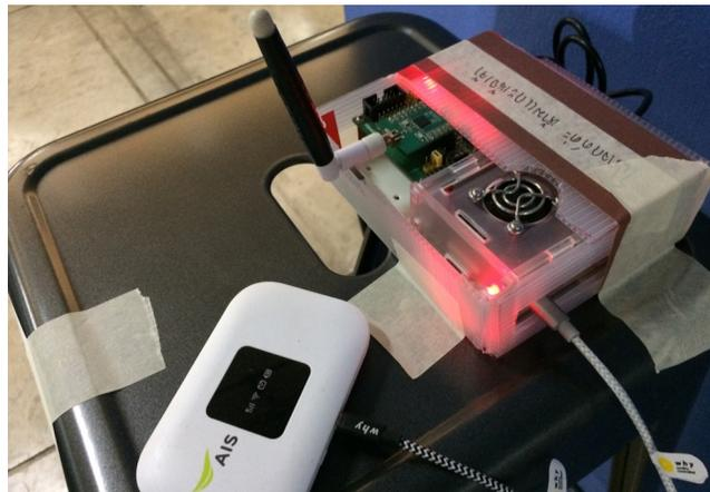
**Figure 8:** Deployed coordinator with cover protection and internet connector.
